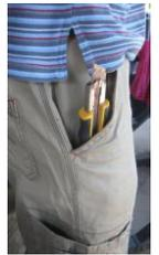
\_\_\_\_\_ carry \_\_\_\_\_ objects in your pocket. This includes tools such as chisels, lathe tools, knives and \_\_\_\_\_. If you fall over you could end up with a \_\_\_\_\_ wound.
