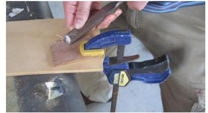
Never attempt a cutting operation while holding the work in your \_\_\_\_\_. The tool will slip and may cut your hand. Always \_\_\_\_\_ the work on the workbench with a \_\_\_\_\_. A \_\_\_\_\_ will provide a support for all cutting operations.
