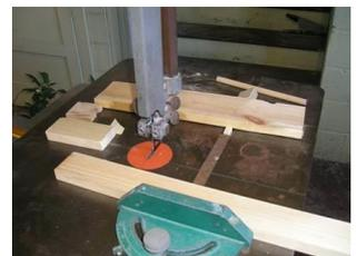
Do not work with clutter on your bandsaw table. A safe bandsaw is a \_\_\_\_\_ bandsaw. Mess as shown in the picture is a \_\_\_\_\_. When you have finished, sweep down the bandsaw table for the next \_\_\_\_\_
