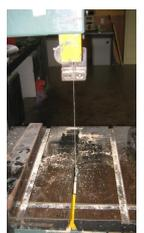
A band saw which is set up in this way is not \_\_\_\_\_(safe/comfortable). The guard is too \_\_\_\_\_(high/low) and exposes the user to a \_\_\_\_\_(cut/burn) injury. If you see a band saw like this, inform your \_\_\_\_\_(teacher/mother) immediately.
